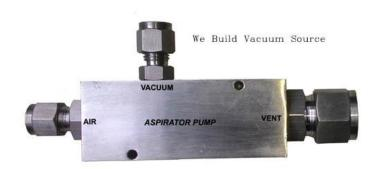
Our simple-to-use aspirator create a strong vacuum for an economical price. The TECHNOSAVVY aspirator features an air/gas suction rate of 12 to 14 liters per minute at its ports, across a series of venturies for quiet, clean, and efficient operation.
